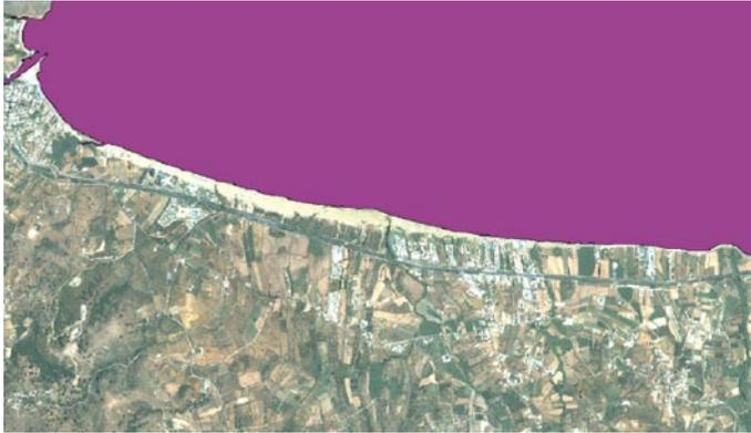
**Figure 11 - The extracted - smoothed polygon corresponding to water.**
