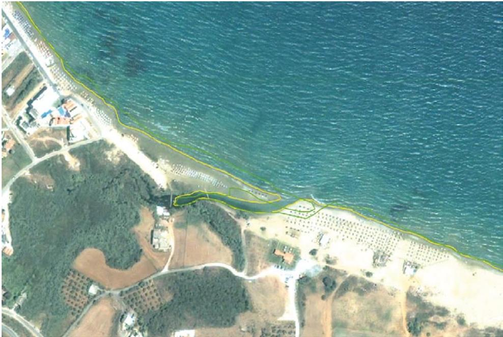
**Figure 14** - Part of the study area as a pseudocolor composition RGB: 3-2-1 of the orthorectified Ikonos image (scale 1:2000). The 1998 Shoreline is shown in green and the 2005 Shoreline is shown in yellow. A shift of about 50m to the ESE direction of the river outflow is observed.
