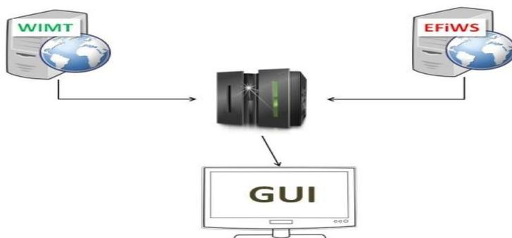
Fig. 1. The distributed architecture. Each component is used via ftp or web service.
