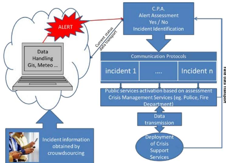
Figure 2: Interface diagram of the services, information systems and databases of the Crisis Management application.
