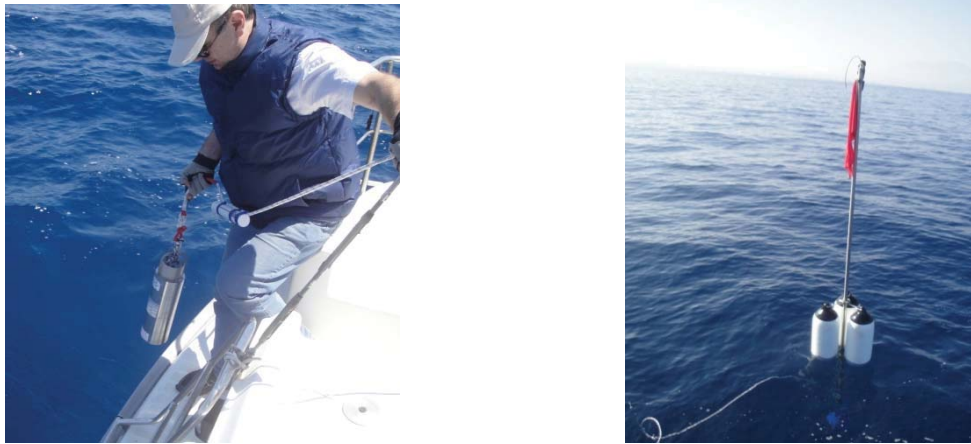
Figure 7: Left: Putting the pinger in the water. Right: The surface float
