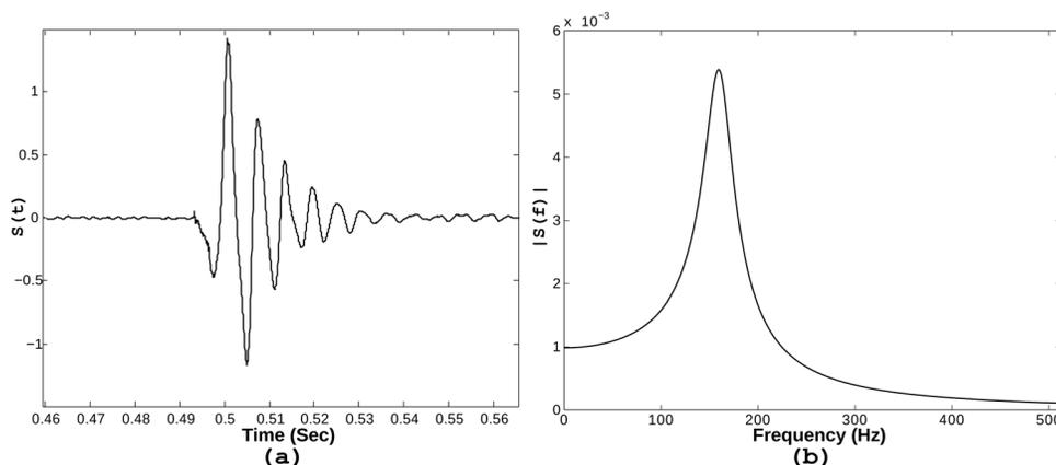
Fig. 1. (a) The actual recorded signal closed to the light bulb source. (b) The simulated signal in the frequency domain.
