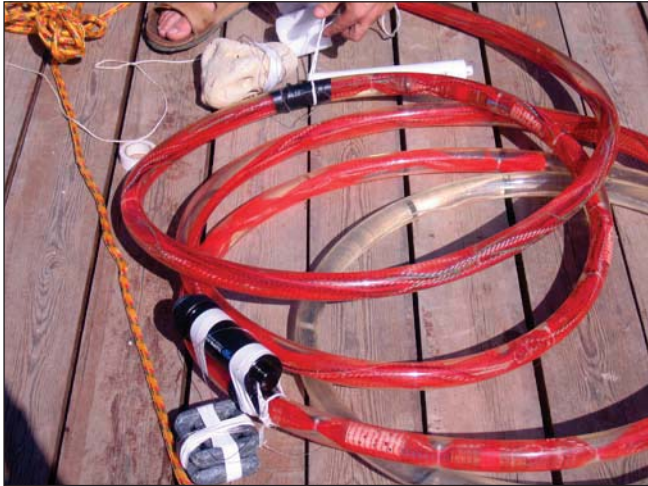
Figure 13. The hydrophone array with the pinger (black cylinder) tied on it.
