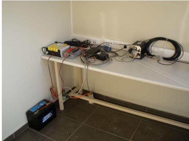
*Figure 2: The inside of the station. The digitizer the Seiscomp computer and the battery that powers the equipment can be seen.*
