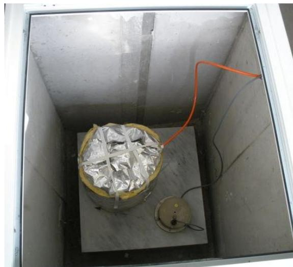
*Figure 1: The well where the seismograph and the accelerometer were placed and insulated. The well was later closed and filled with insulation material in order to keep the temperature inside the well constant*
