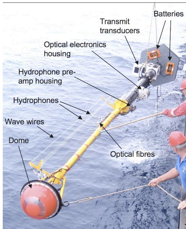
Figure 1. A labeled photograph of the buoy as it is deployed.
